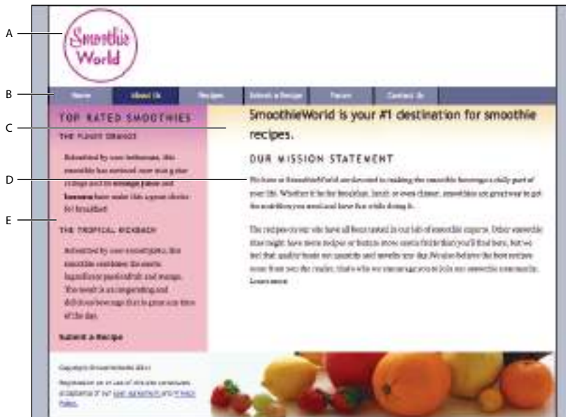
The structure of your SmoothieWorld site with HTML5 elements A. Header. B. Nav. C. Section. D. Article. E. Aside.
