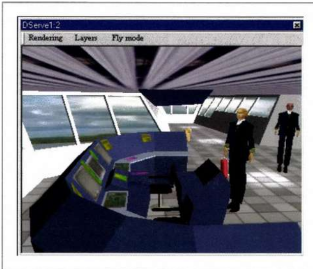
Figure 8.14 The virtual bridge in a training simulator
