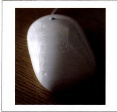
Figure 2.10 A Mac one-button mouse. The single button of the traditional Mac is said to have the advantage of ‘you always know which button to press’
