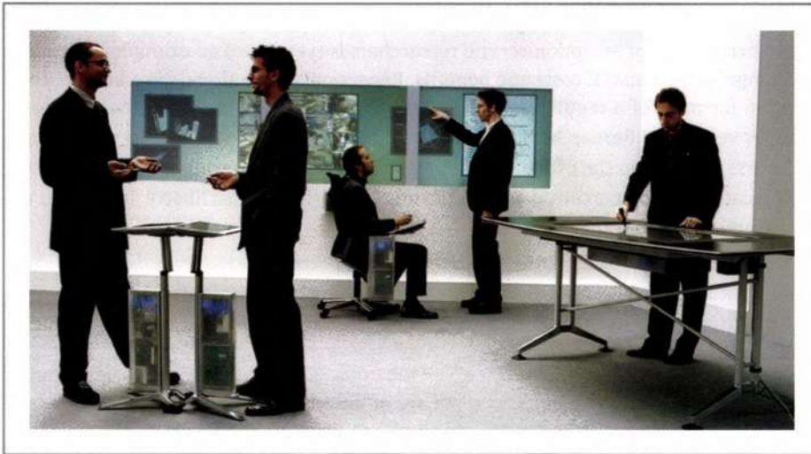
Figure 16.9 The second generation of the IPSI Roomware components (DynaWall, InteracTable, CommChair, ConnecTables) developed in 1999
