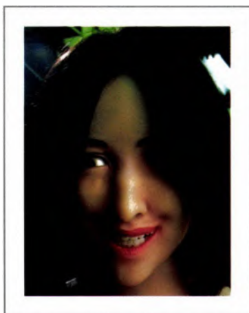
Figure 24.3 Female face robot: smiling third-generation female face robot. Inside this robot's head is a CCD camera which it uses to gather visual stimuli. It will react to stimuli with a facial expression based on one of six basic emotions (anger, fear, disgust, happiness, sadness, surprise). Unlike previous generations, this robot can interact with humans in real-time. Previous generations had taken too long to form and lose a facial expression. This robot face was developed at the Laboratory of Fumio Hara and Hiroshi Kobayashi at the Science University, Tokyo, Japan.
