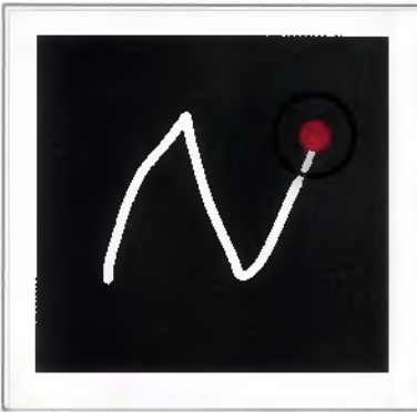
Figure 13.12 The N-wave gesture to open a browser; the red and black circles give feedback on the user's touches
