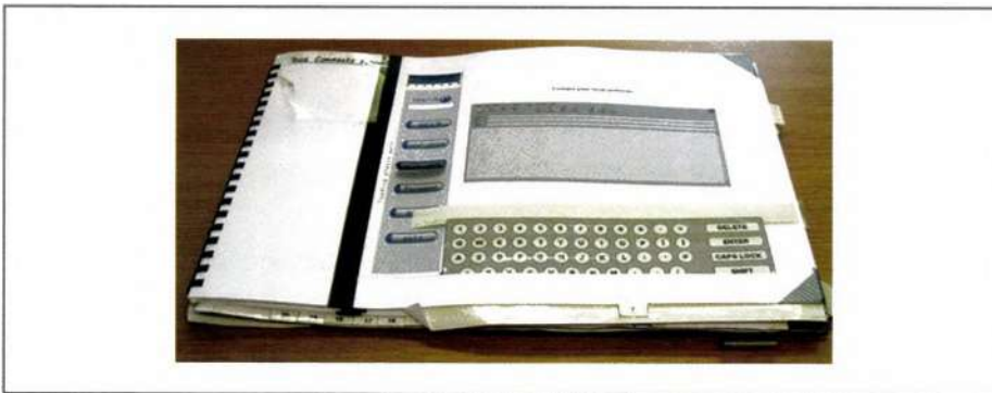
Figure 8.9 Paper prototype of a messaging screen for a home communications centre (Source: David Benyon)
