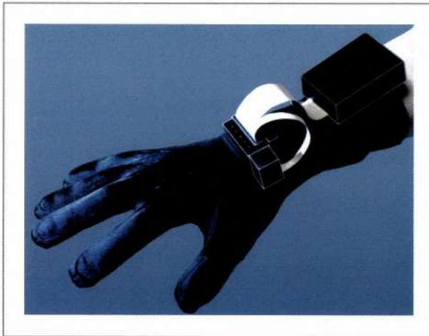
Figure 13.6 A force-feedback data glove
