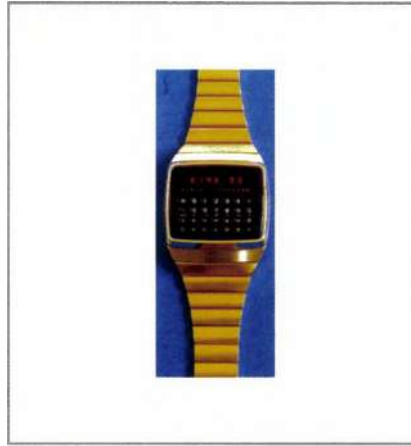
Figure 20.5 The HP-01 algebraic watch
