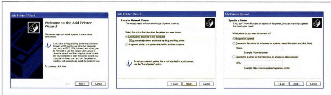
Figure 21.10 Using a Microsoft wizard to prompt a user to supply information one step at a time
